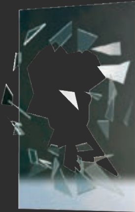
Annealed Glass Breaks easily, producing long sharp splinters
